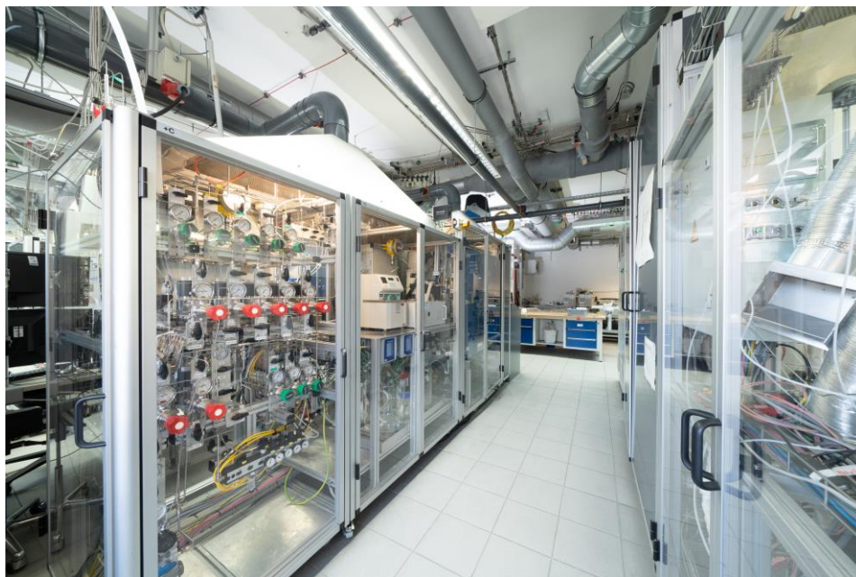
Figure 1: 16-fold high throughput system customized for HCl chemistry
