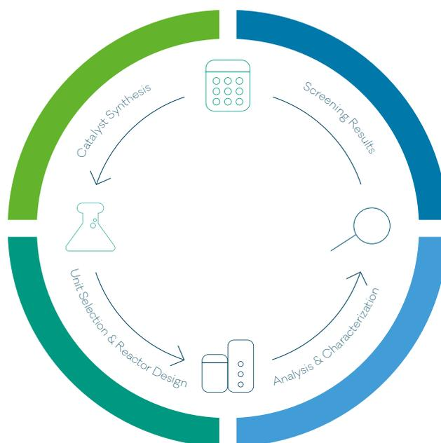
Figure 3: Development cycle for producing 16HD from C6 polyols. The catalyst scale-up in this example involves shell impregnation of commercial carriers. The product analysis involves detailed GC-MS and GC-FID/TCD analysis identifying more than a hundred compounds within the reaction network. The testing comprises HTE as well as flexible bench-scale equipment.
