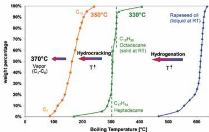
Simulated Distillation of reaction products at different temperatures
