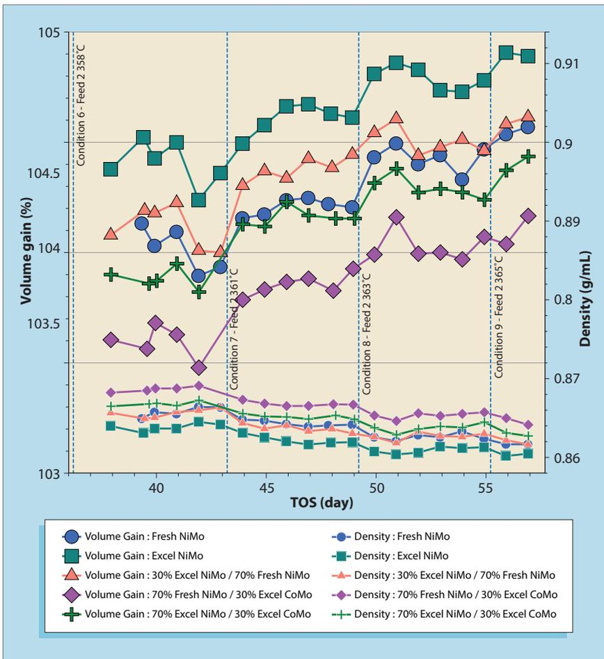
Figure 6 Volume swell for all catalyst configurations
