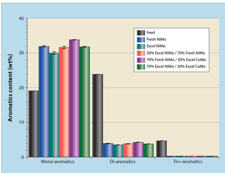
Figure 5 Aromatics content in feed and products for condition 9
