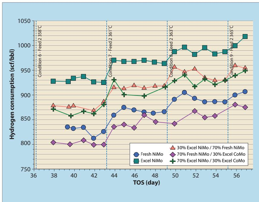
**Figure 8** Hydrogen consumption for all catalyst configurations
