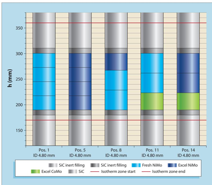
Figure 1 Loading configurations of fresh and rejuvenated catalysts
