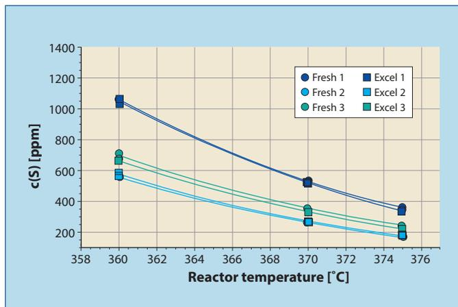
**Figure 2** Product sulphur vs temperature for catalyst configurations tested at 80 barg
