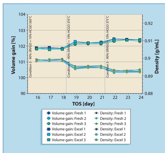
**Figure 7** Volume gain for catalyst configurations tested at 80 barg
