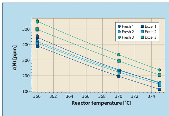
**Figure 5** Product nitrogen vs temperature for catalyst configurations tested at 120 barg
