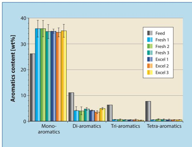
**Figure 6** Aromatics content for catalyst configurations tested at 80 barg and 370°C
