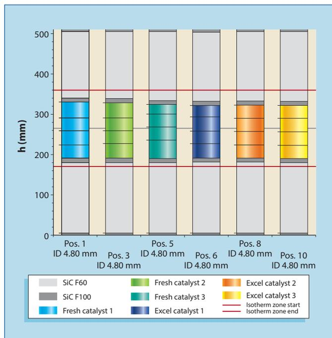
**Figure 1** Loading configurations of fresh and Excel rejuvenated configurations
