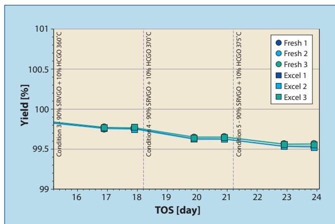
**Figure 9** C<sub>5</sub>+ yield for catalyst configurations tested at 80 barg
