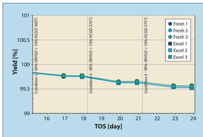
**Figure 10** C<sub>5</sub>+ yield for catalyst configurations tested at 120 barg
