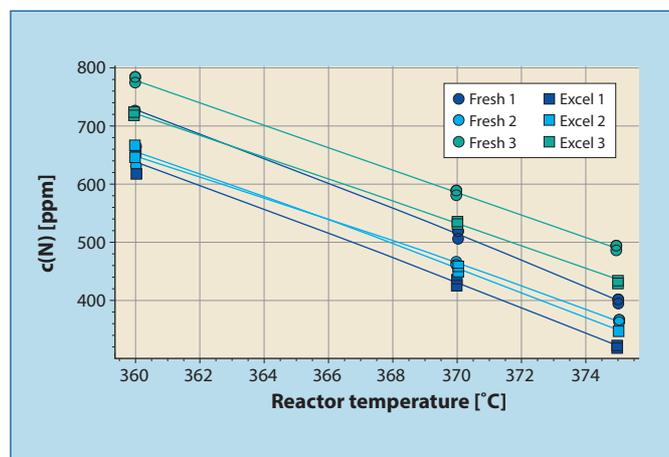
**Figure 4** Product nitrogen vs temperature for catalyst configurations tested at 80 barg
