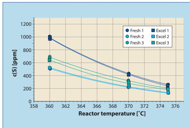
**Figure 3** Product sulphur vs temperature for catalyst configurations tested at 120 barg
