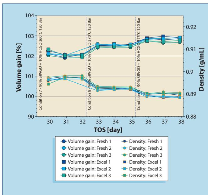
**Figure 8** Volume gain for catalyst configurations tested at 120 barg
