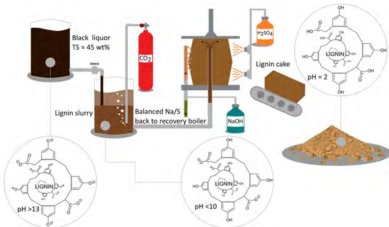
Figure 2. Lignin precipitation.
