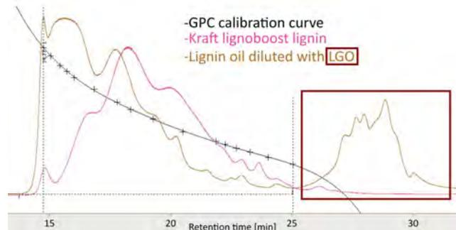
Figure 4. Gel-permeation chromatogram of Kraft Lignoboost lignin and lignin oil/feed mixture.
