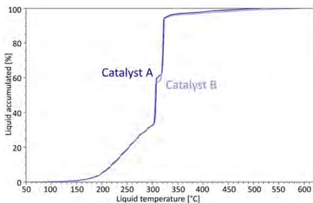
Figure 7. Simulated distillation of liquid fraction of day 8.
