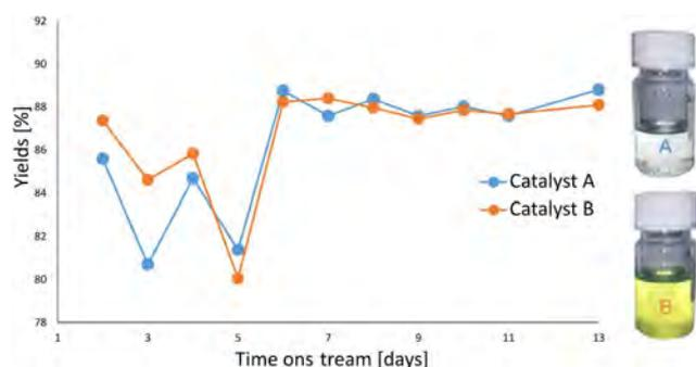
**Figure 6.** Liquid recovery generated by hydrotreatment of the lignin/TOFA/LGO feed for a period of 13 days (300 h) on stream. The yields for samples A (blue) and B (orange) are given, the boiling range is 180–345 °C. The yield is based on the overall hydrocarbon outcome as obtained by simulated distillation (ASTM D7213).
