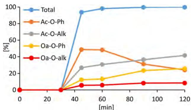
**Figure 5.** Esterification of KL with  $^{13}\text{C}$ -labeled oleic acid and acetic anhydride over time. Relative abundances are given for aromatic acetates (Ac-O-Ph), aliphatic acetates (Ac-O-Alk), aromatic oleates (Oa-O-Ph), and aliphatic oleates (Oa-O-Alk).
