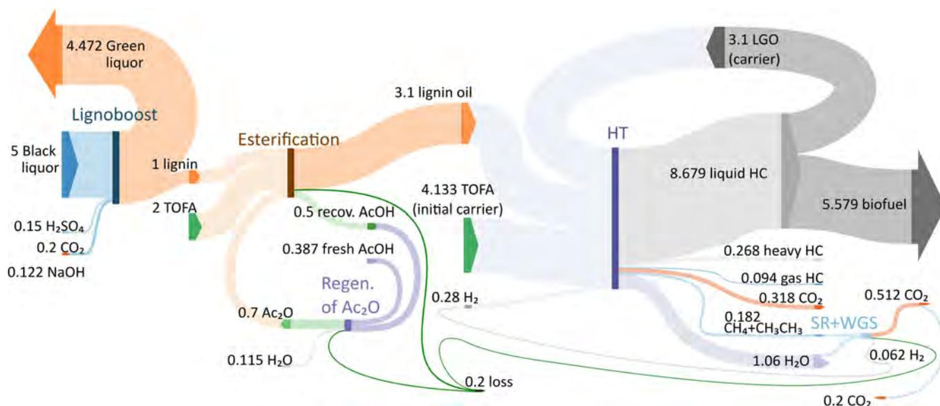
**Figure 8.** Sankey diagram of the overall process.
