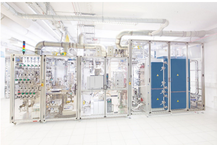
Figure 1: Flexible 16-fold parallel high-temperature test system
