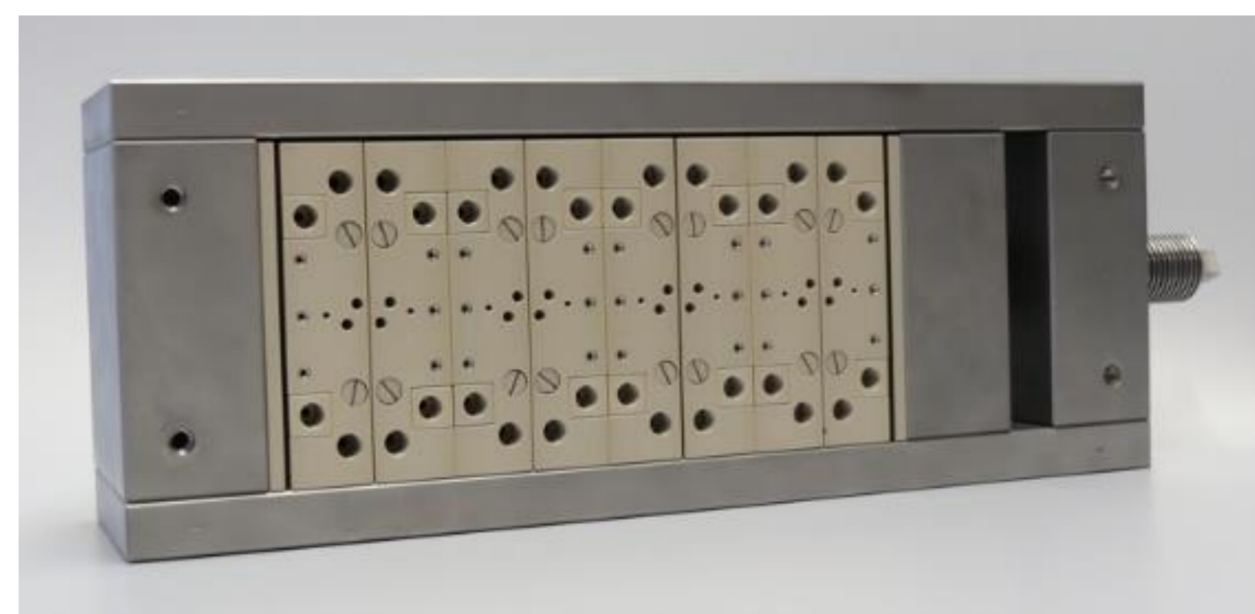
Figure 3: Mechanical press with four flow cells
